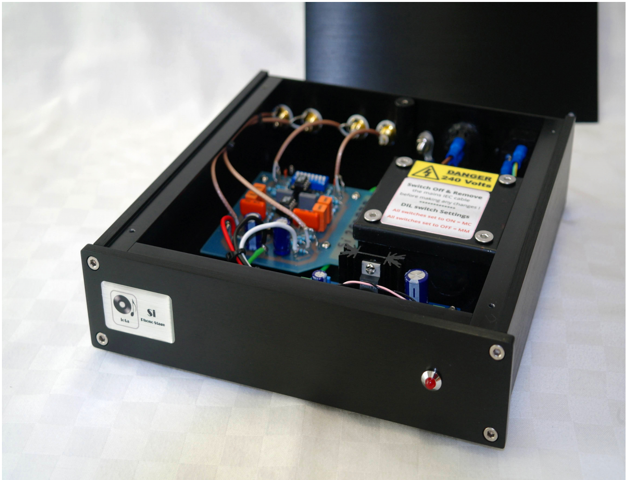
iota Si Phono Stage internal view
